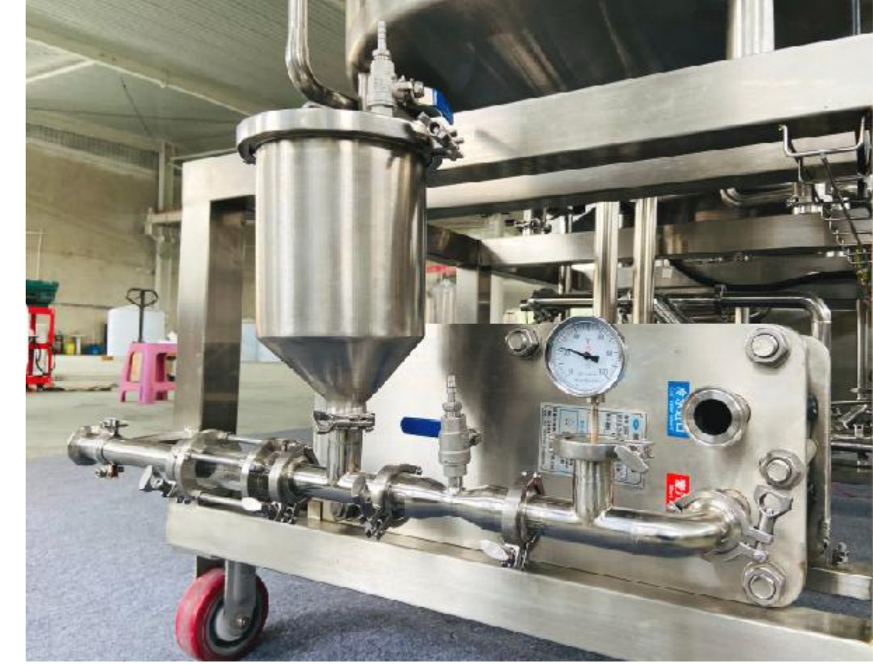
Yeast adding tank - recommended only if temperature out of PHE can be controlled under 30°C or less
