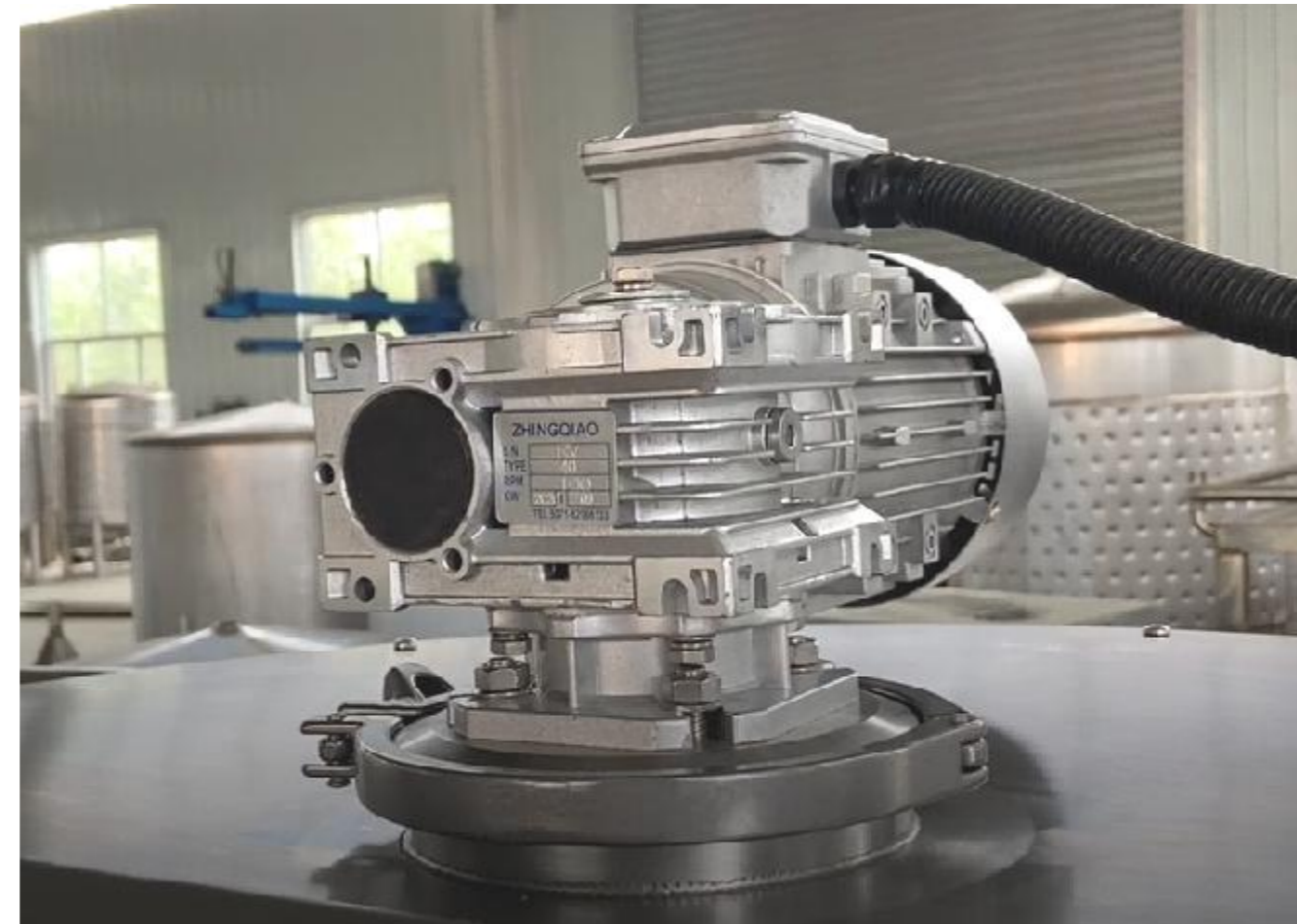
VFD Speed control grain raker - mounted on top of lid of mash tun, with 0.55KW motor & reducer
