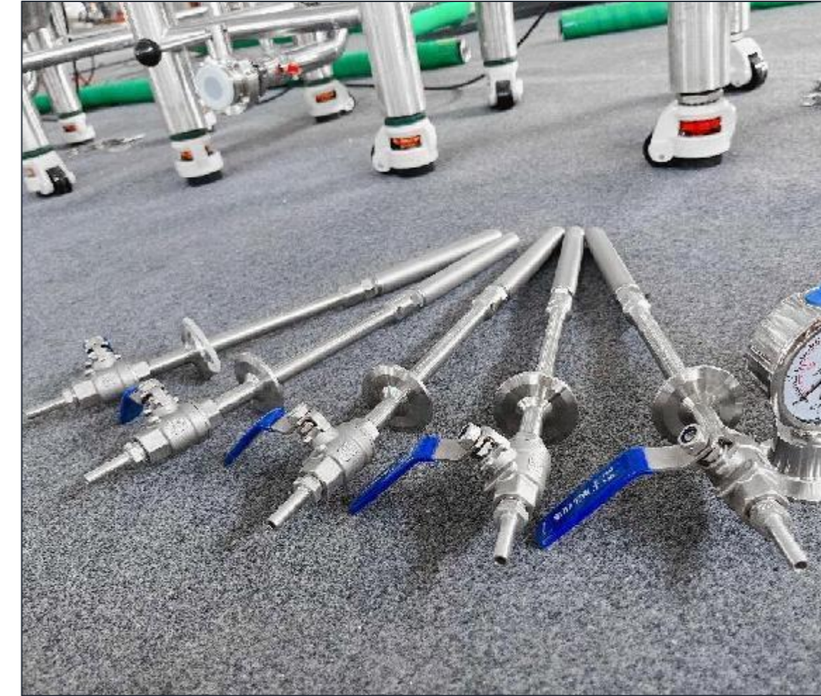
Spunding Valve to replace the pressure relief valve
