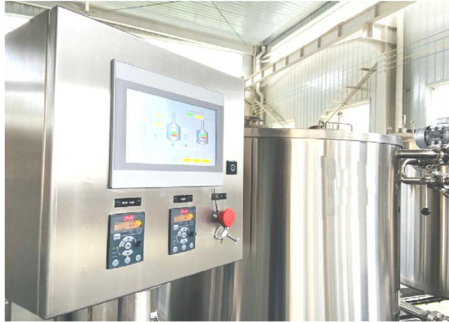
PLC Control System - Programmed, can save mashing temperature for different recipes
