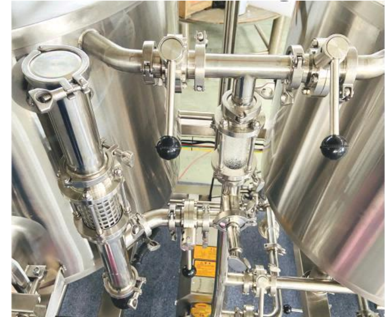
RIMS Set-up outside of mash tun - 5kw Electric heating elements built inside of the pipe, for multiple-steps mashing requirement, power on/off to be controlled from PID system
