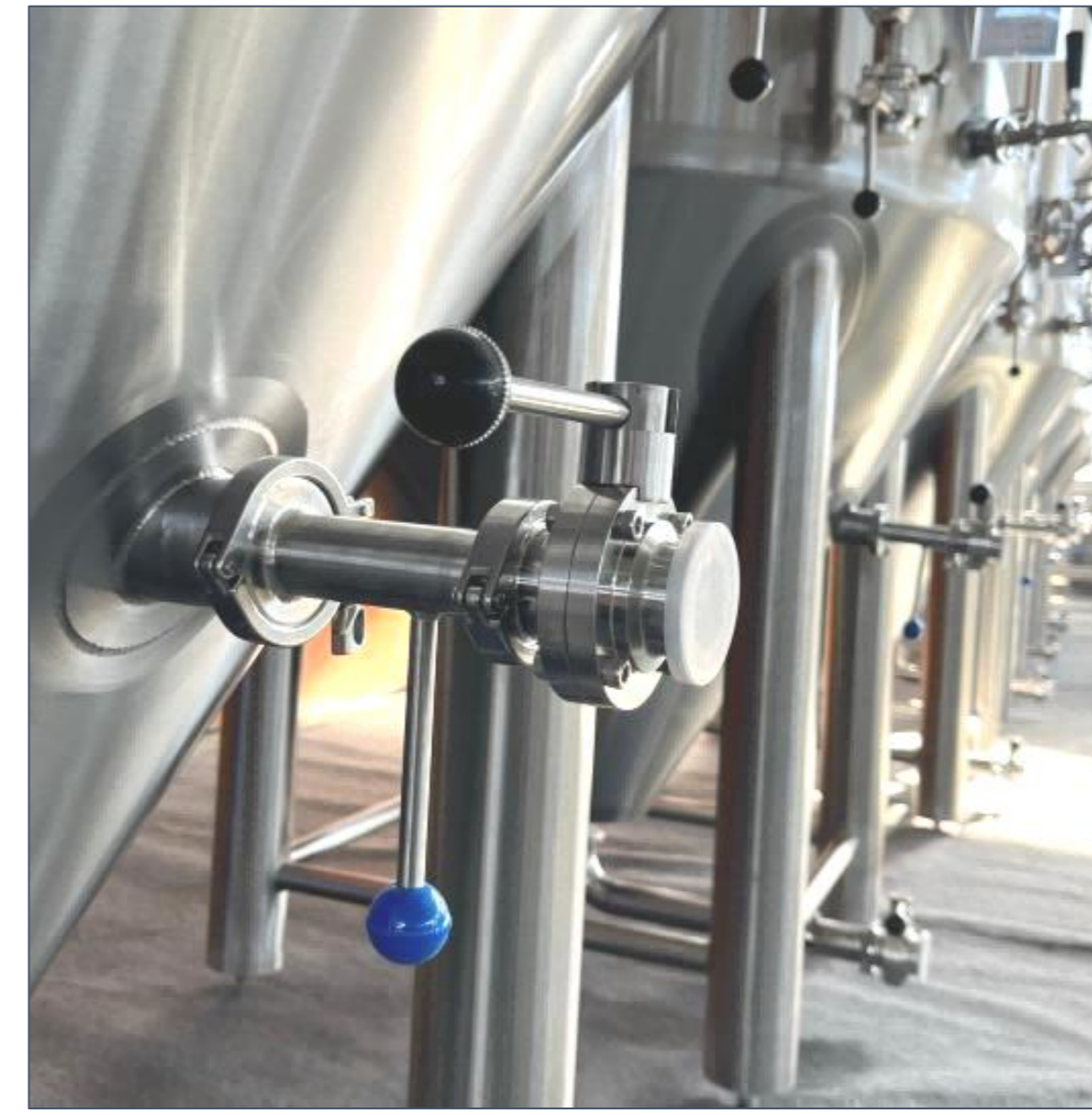
Higher quality sample valve with sampling coil
