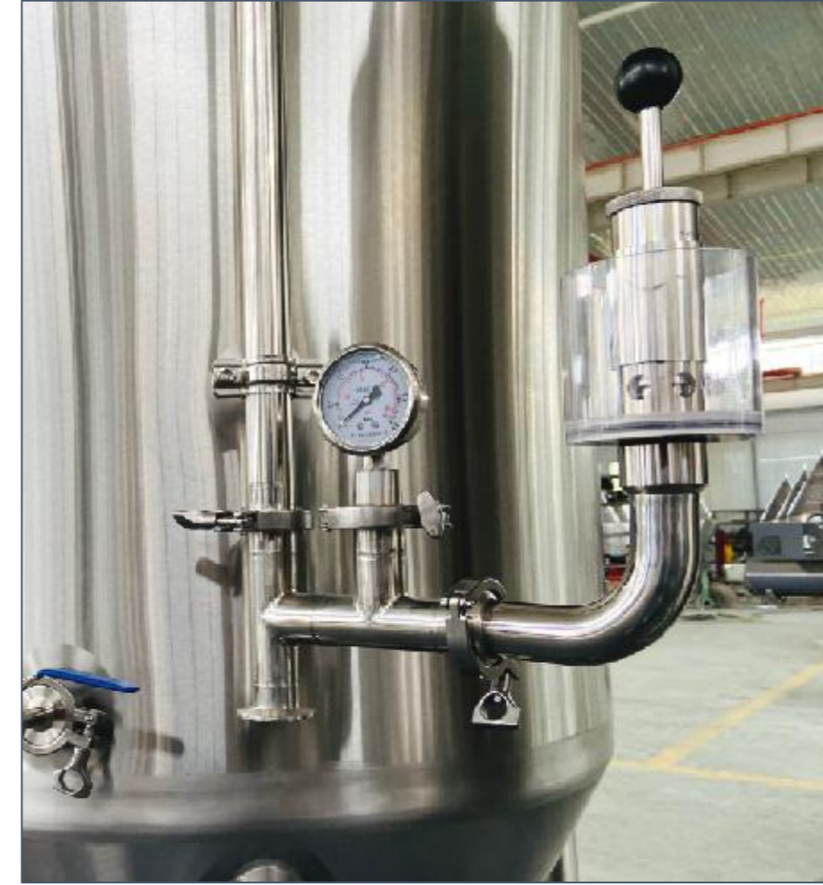
Spunding Valve to replace the pressure relief valve
