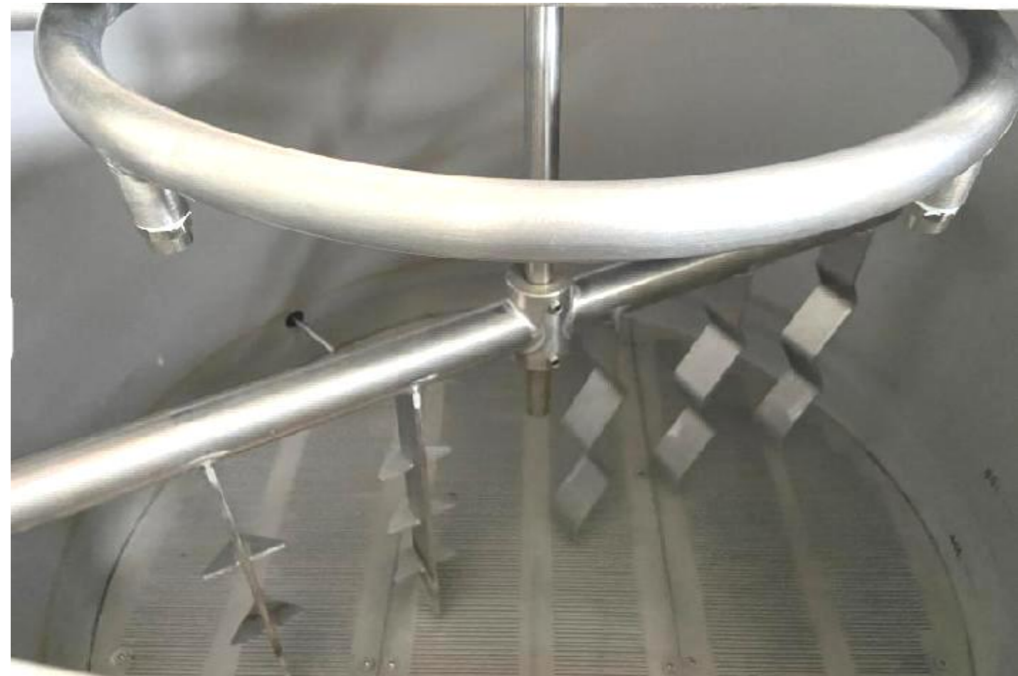
VFD Speed control grain raker - mounted on top of lid of mash tun, with 0.55KW motor & reducer
