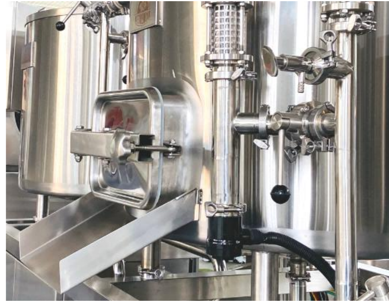
RIMS Set-up outside of mash tun - 5kw Electric heating elements built inside of the pipe, for multiple-steps mashing requirement, power on/off to be controlled from PID system
