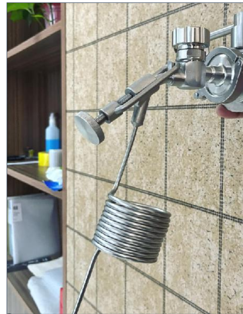
Dry hopping device to add hops without oxygenation under pressure
