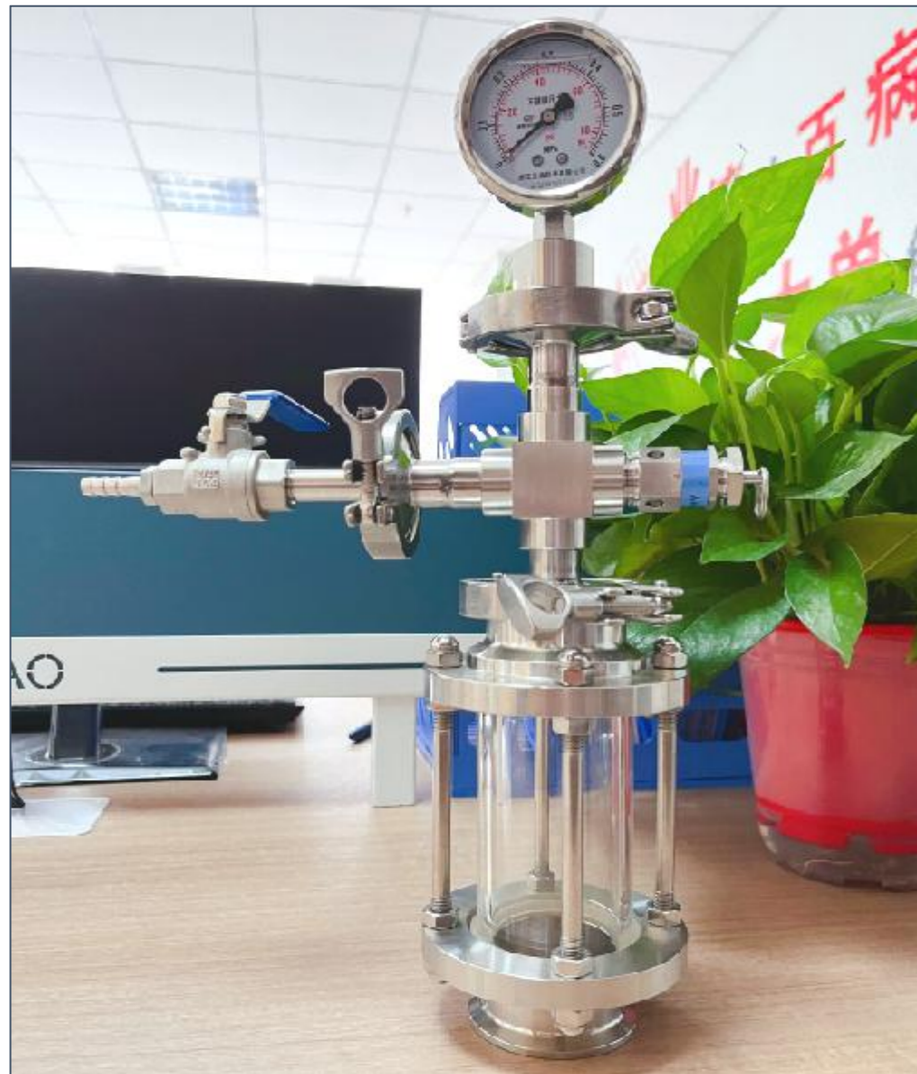
Dry hopping device to add hops without oxygenation under pressure
